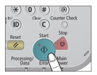
If the following screen appears, press  $\odot$  (Start) to scan the next original. After all of the originals are scanned, press [Start Sending].
